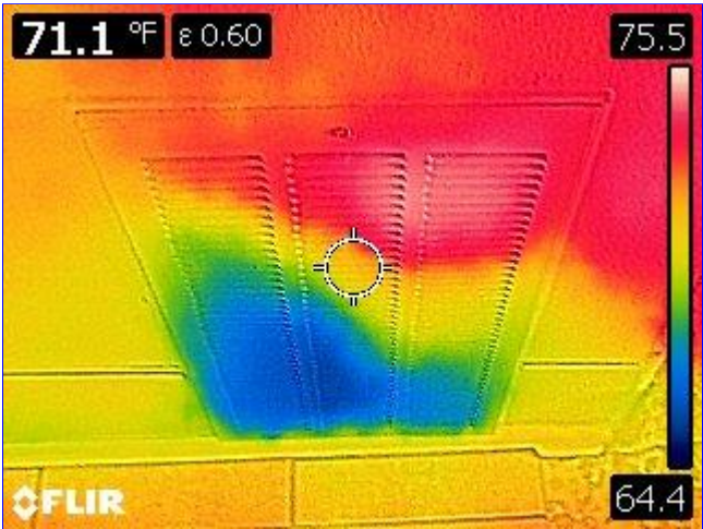
C. Item 4(Picture) Only a 6 degree difference between the return air and supply ducts in living room. Ducts possibly crimped.
